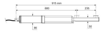
HINDI 880 SPRINT is an oil-hydraulic actuator particularly recommended for swinging gates up to 2.3 meters, each gate leaf. It is very simple to install by means of two plates and bolts to be fixed to the gate and gate post respectively, allowing the opening and closing of the gates.
