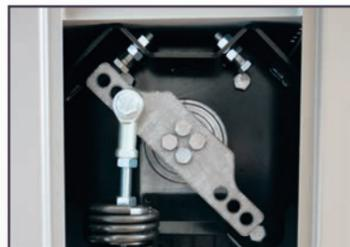
Springs are available in different types according to the length of the arm and are certified for millions of operations. The mechanical balancing system is enhanced by the use of adjustable mechanical stops.
