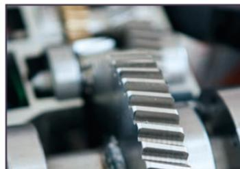
The motor and all of the gears are produced and manufactured in the **Roger Technology** factories. They are rigorously tested and manufactured in steel and bronze with helicoidal teeth which are angled at 15 degrees to ensure perfect movement during operation.
