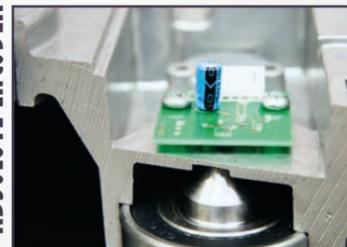
Powerful, innovative and precise, the absolute encoder is assembled on the slow shaft of the motor. The barrier will start perfectly after a power failure or if manually released, without the process of re-learning.
