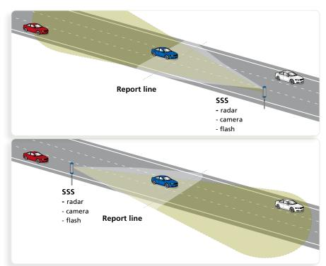
The SSS operates from the side of the road, tracking traffic for speed and distance.
